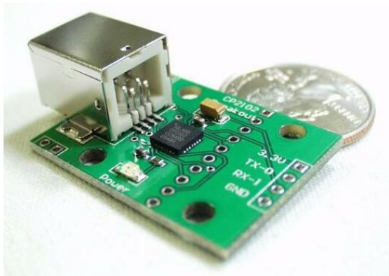
Photo 10: CP2102 USB-to-TTL interface from SparkFun
