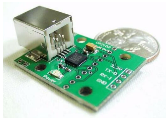
Photo 10: CP2102 USB-to-TTL interface from SparkFun
