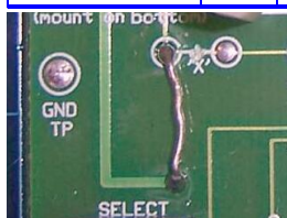
Photo 2: Adding 5V to P4 (See Assy step 8)
