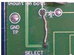
Photo 2: Adding 5V to P4 (See Assy step 8)
