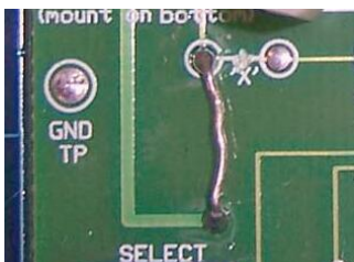
Photo 2: Adding 5V to P4 (See Assy step 7)
