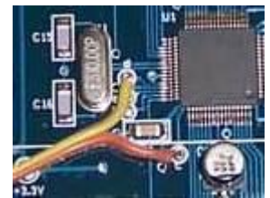
Photos 1a and 1b: "Extra Signals cable" (See Assy step 6) (Photo 1a shows 3 wires, but only two wires used now.)
