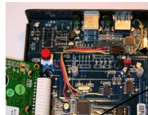
Photos 1a and 1b: "Extra Signals cable" (See Assy step 6) (Photo 1a shows 3 wires, but only two wires used now.)
