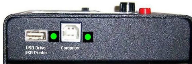
NUE-PSK modem with the USB ports accessible on the left side of the enclosure
